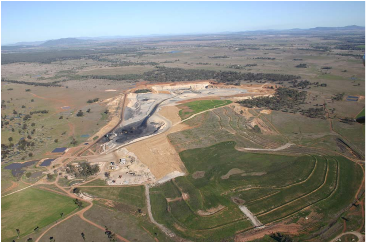
Plate 1: An aerial view of the Whitehaven Coal Mine showing contour banks and rock-lined waterways on the rehabilitated post-mining landform (Ref. E513-134.JPG)
