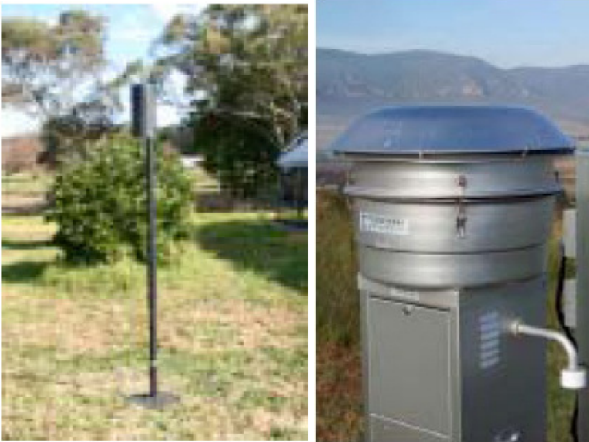
Deposited Dust and High Velocity Air Sampler.
